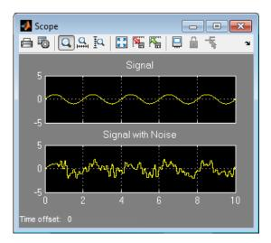
You have now built a digital filter and used it to model the presence of colored noise in your signal. This is analogous to modeling the low frequency noise reaching the microphone in the cockpit of the aircraft. Now that you have added noise to your system, you can experiment with methods to eliminate it.
